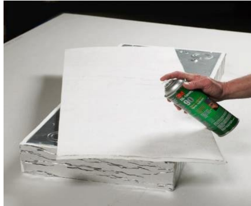
Adhesive, installing and adhering to back of box
