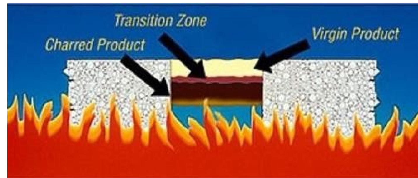
As fire intensifies, a hard char with thermal insulation is formed.
