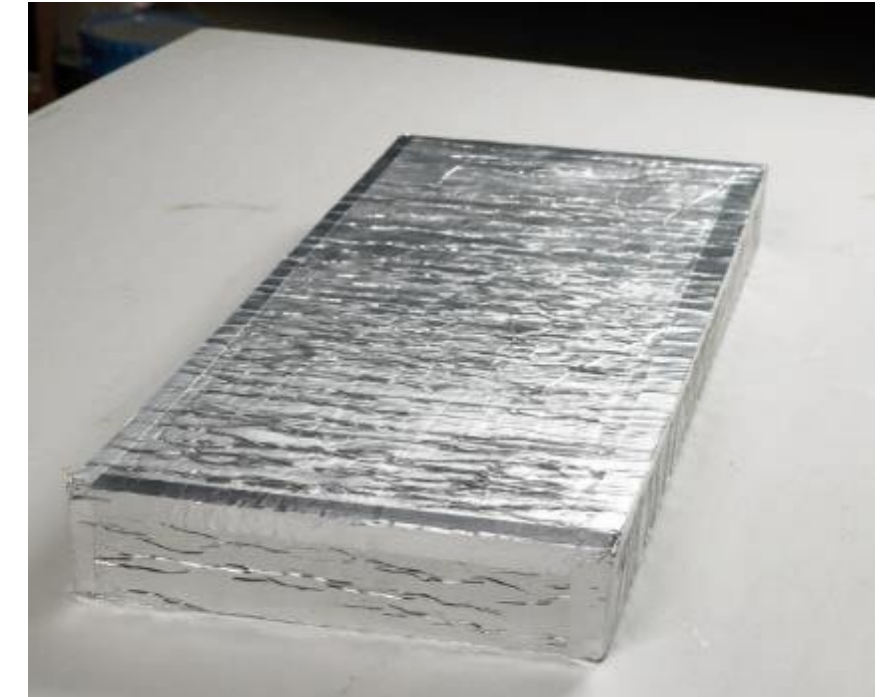
Sealing all mat interfaces with aluminum foil tape
