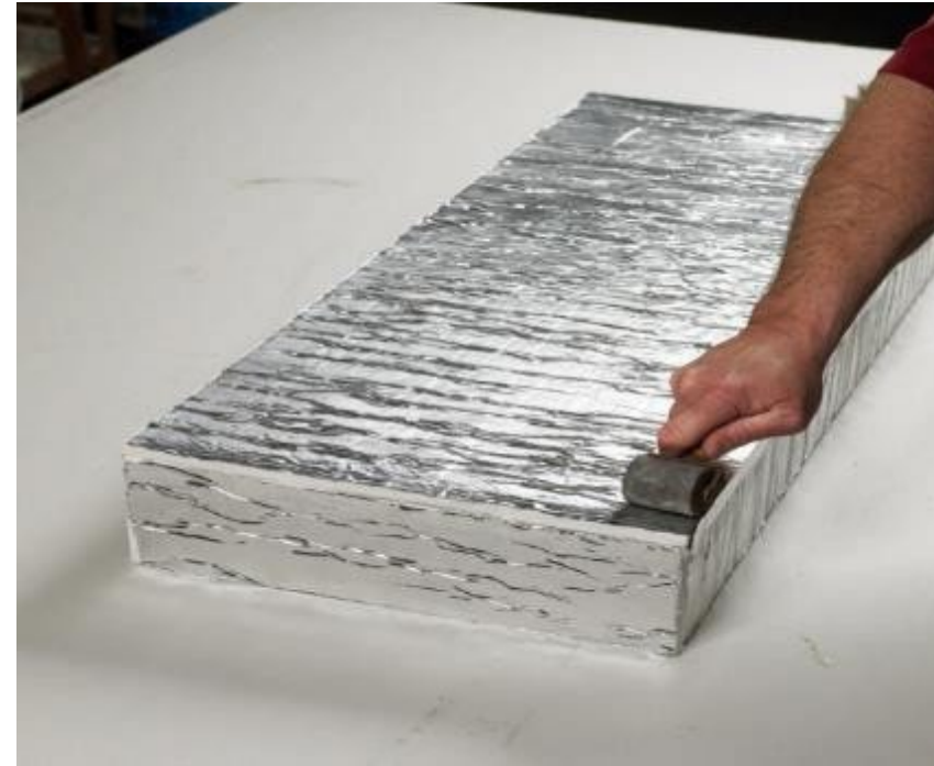
Adhesive, installing and adhering to back of box
